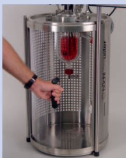
Polycarbonate protection door for optimal user safety
